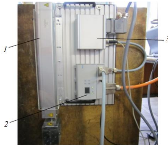
Fig. 1. General view of the experimental installation of a mechatronic module with a linear motor, for the performed technological linear movement of structural units of group packaging: 1 – a linear motor; 2 – controller; 3 – feedback system.
