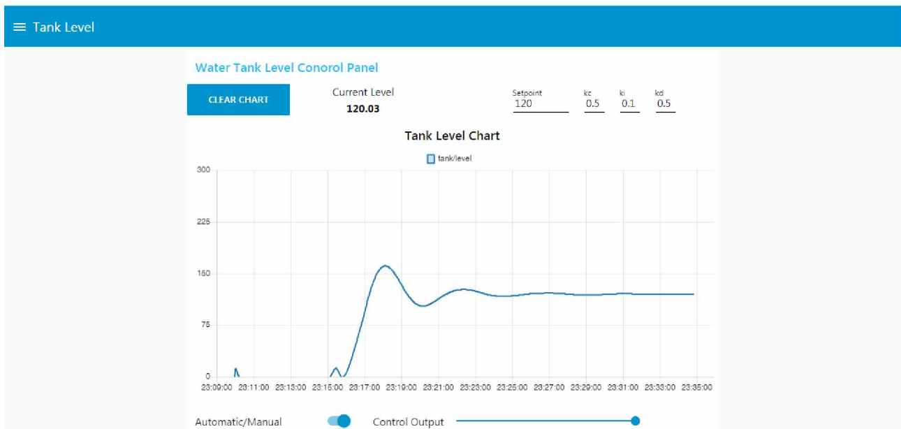
fig.7 Tank Level control Panel
