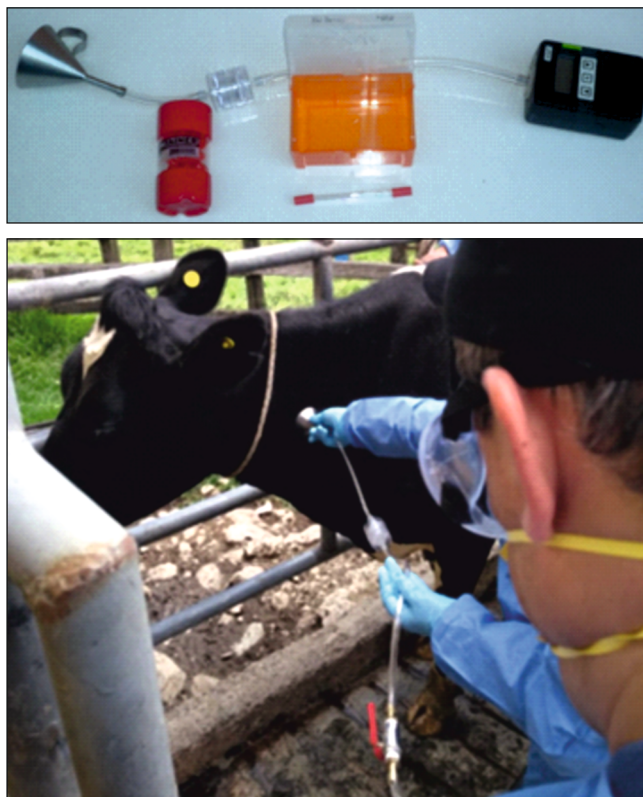
Fig. 1. The sampling of VOCs emitted through the skin of farm cows
