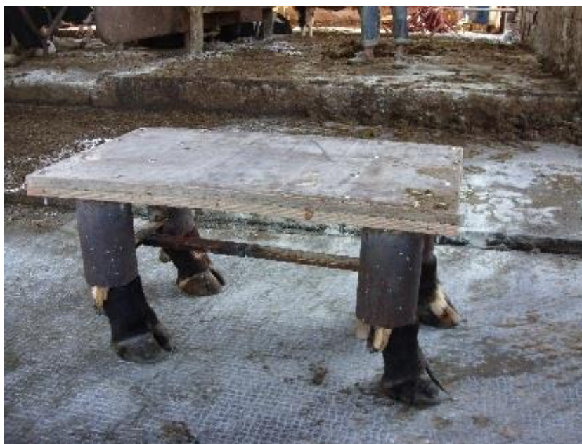
Fig. 1. Tribometer for determination of coefficient of friction between the hooves and the floor (Philips and Morris, 2000).
