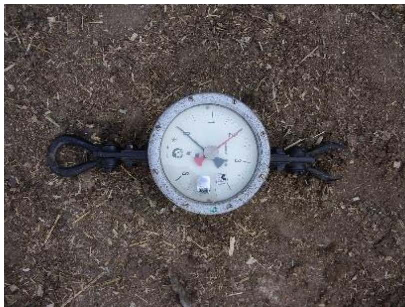
Fig. 2. Dynamometer for measuring applied force
